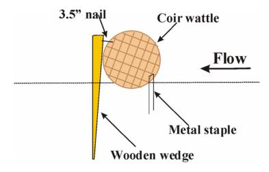
Figure 10 Installing coir wattles with wedges and staples.
