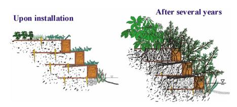
Figure 7 Conceptual diagram of coir block application.
