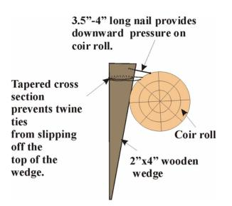
Figure 8 Installing coir logs with wedges.
