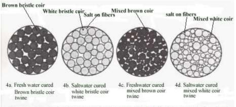
Figure 4. Enlarged cross section of currently available different types of coir twines
