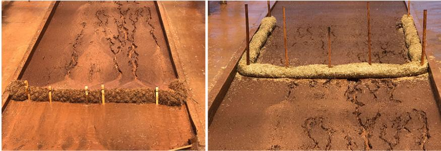
Figure 2: Field experiment showing the superior performance of RoLanka's BioD-Wattl coir wattles than straw wattles with synthetic netting.
