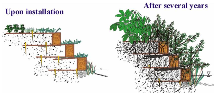
**Figure 7 Conceptual diagram of coir block application.**
